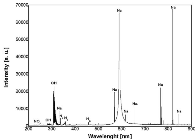
**FIGURE 5** The emission spectrum of dc-APGD generated in contact with the flowing liquid cathode (0.85% NaCl)
